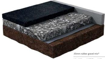
Min 100mm MOT Type 1 20mm to dust (non-recycled), Laid, level and compacted to the required tolerance.
