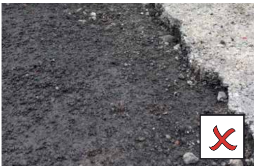
EDGES ARE NOT CLEAN AND DURABLE. THIS MAY PREVENT A COHESIVE BOND
