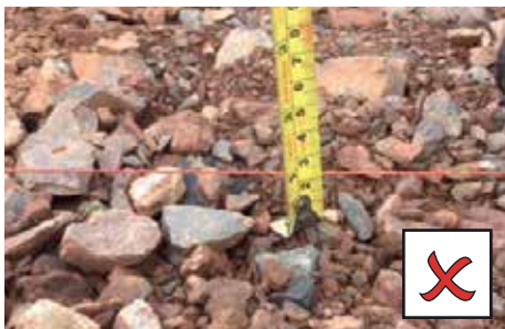
UNDULATIONS ARE GREATER THAN 10MM
